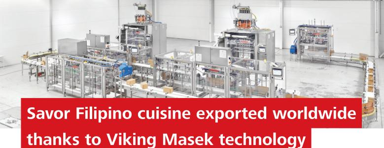
Recently Viking Masek installed the first of multiple packaging lines at the largest Filipino manufacturer of spices and sauces - Mama Sita's ®. The complete packaging line consists of two (2) sachet machines SA600, each of them producing 250 sachets/min, and a top load cartoning system with carton erector CFM, loading units and carton closer CLM.
